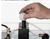
Ultrasonic thickness measurements are accurate, reliable, and repeatable. Instant readings can be achieved from one side of a material, making it unnecessary to cut up or destroy the part.
